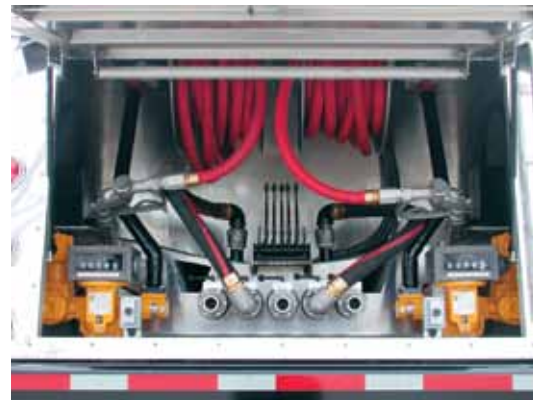
Photo above shows 2" ends used on jumper hoses and 1-1/2" ends on reel fuel delivery hoses.
