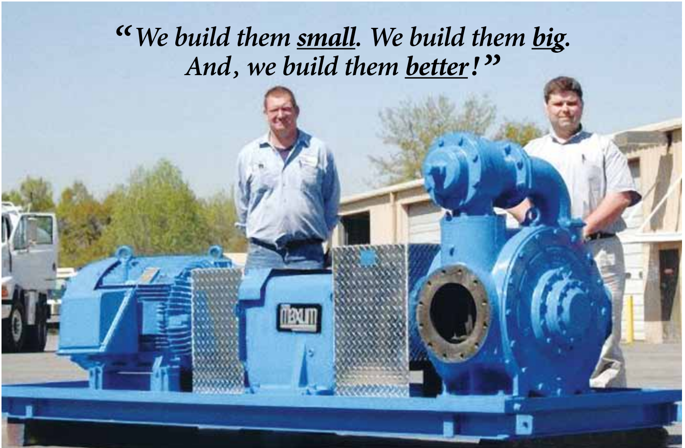
Shown in photo above: Blackmer Pump, HXL-12, 100 HP, 2200 GPM
